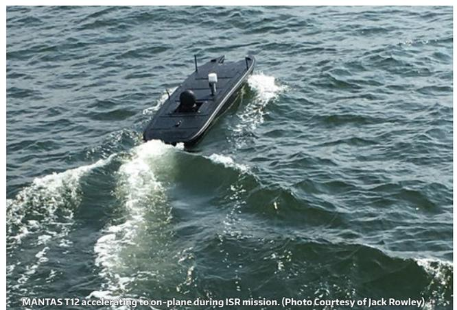
a MANTAS USV was used to conduct inspections of the Keokuk dam and energy center, the Bagnell energy center, the Elkhart hydro dam, the Central Arizona Project canal and other infrastructure.
