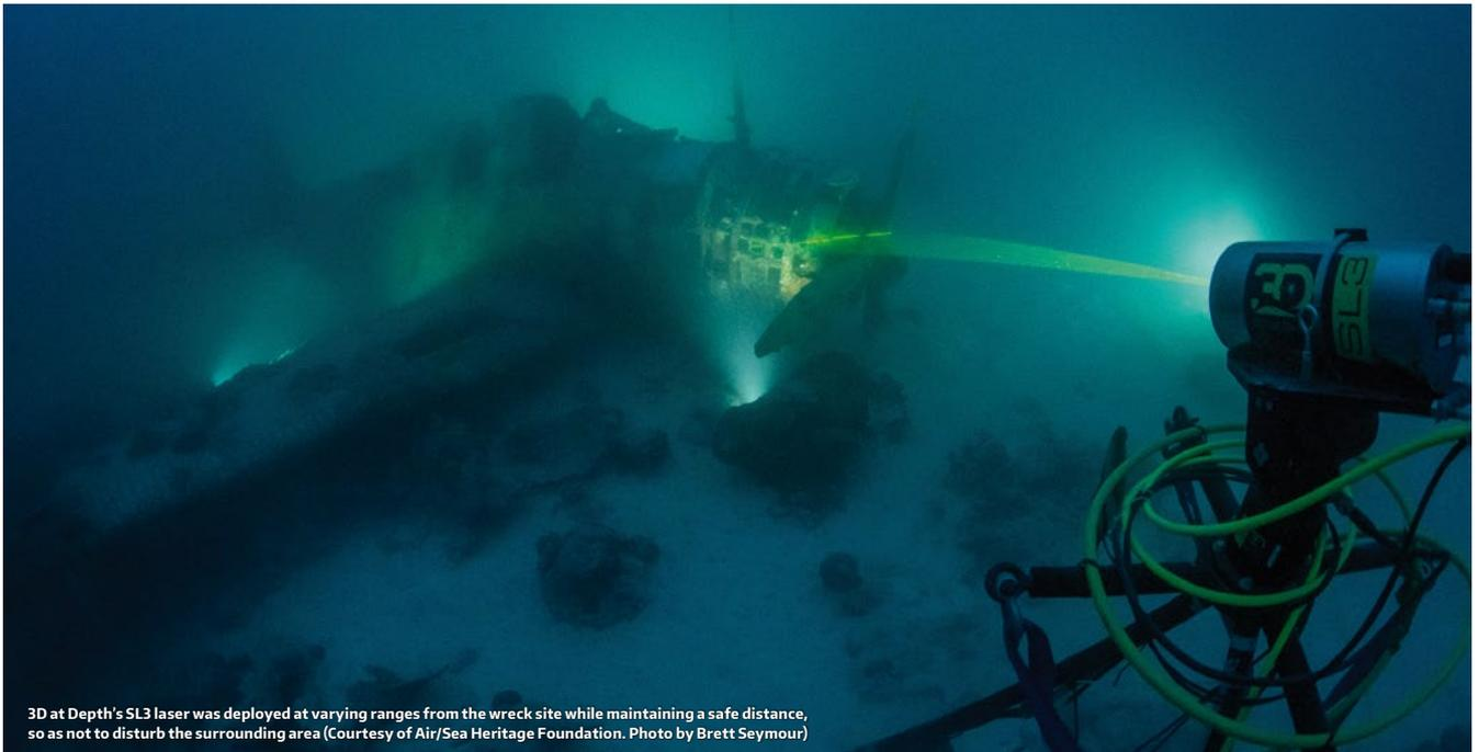
3D at Depth's SL3 laser was deployed at varying ranges from the wreck site while maintaining a safe distance, so as not to disturb the surrounding area (Courtesy of Air/Sea Heritage Foundation. Photo by Brett Seymour)
